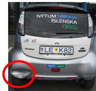
Figure 11: the Icelandic Mitsubishi iMiEV, red circle indicating the damaged impact area.
