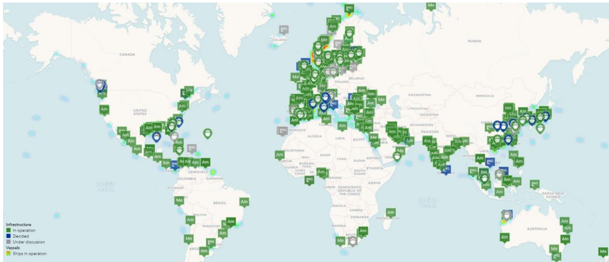
Figure 5 Bunkering infrastructure in operation and decided for ammonia, LNG and methanol in 2022 (DNV, 2022)
